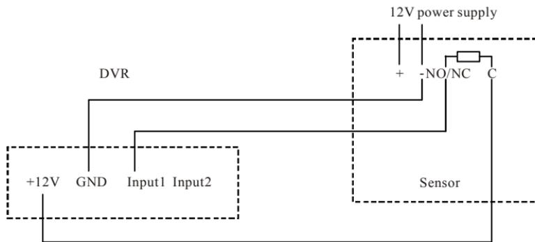
If we parallel connected the sensor, the DVR can not recognize the triggered sensor. User need to have a resistance.
