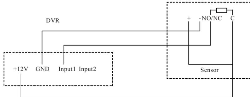
If the distance between the probe and DVR is too far, the probe requires a separate power supply:
