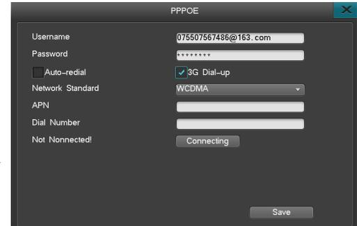
A. Make sure whether your 3G network card are belong to one of HUAWEI's EC1260\EC1261\EC122\E261\E353\E153 model, because, this NVR software can only support these type of 3G.
