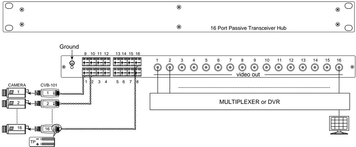
CVB-216 is a multi video transceiver designed for one compact 19" wide 1U panel. Panels can reside in the same rack as other equipment, such as switchers, multiplexers, DVR, video conferencing equipment, etc. It's perfect for larger CCTV installations and ideal for security monitoring stations.
