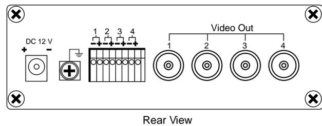
Use CVB-204 4 channel passive video transceiver as transmitter to work with active CVB-404 receiver for transmission range of 3200 feet. Use CVB-301T transmitter to work with CVB-404 for transmission range of 4900 feet with a color signal or 7800 feet with a B/W signal.
