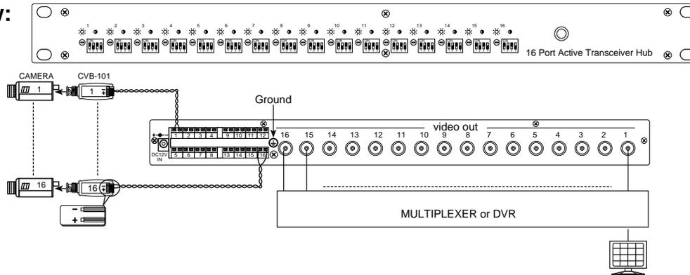
CVB-416 is an active video receiver designed for one compact 19" wide 1U panel. Panels can reside in the same rack as other equipment, such as switchers, multiplexers, DVR, video conferencing equipment, etc. It's perfect for larger CCTV installations and ideal for security monitoring stations.
